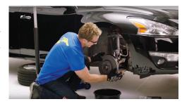
Install a lugnut on the top stud finger-tight to keep the rotor in place. Lubricate your cleaned or new caliper hardware with a high-temperature brake parts lubricant, also available where you bought the solvent. Use a gloved finger to apply the lubricant. You need only a smear on each moving surface and guide pin; if you overapply the lubricant, there is a risk it could leak onto the braking surface of the pad and rotor and contaminate the brake pad, reducing its effectiveness.
