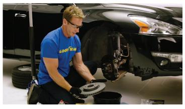
of any of these problems. If they're damaged or worn down, detach the rotor from the wheel studs. If there's extensive rust buildup, you might have to give it a whack with a hammer to loosen it. Then swap in the new rotor and replace the assembly.
